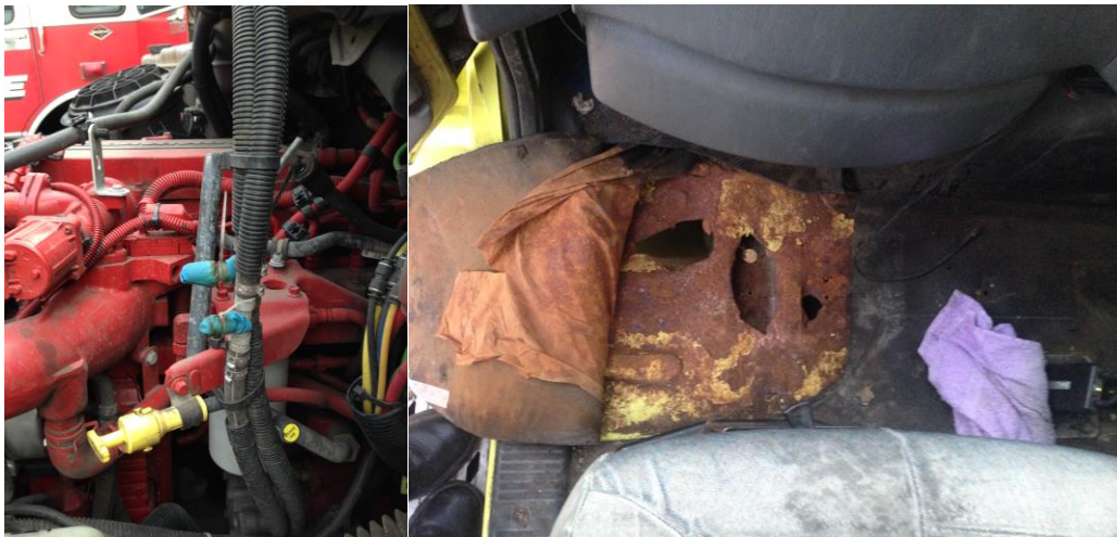
LEFT: gloves and plastic ties are used to repair an engine. RIGHT: Rust holes in the floorboards of X7.
